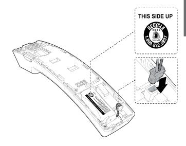
4. To replace the handset cover, align all the tabs on the handset cover against the corresponding grooves on the handset, then firmly push downward until all the tabs lock in the grooves. Then install the screw.
