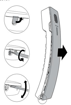
2. Unplug the battery connector from the socket and then remove the battery from the handset battery compartment.
